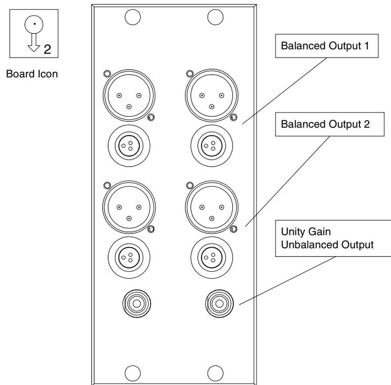
**Figure 7: Spirito Reference Output Card Connectors**
