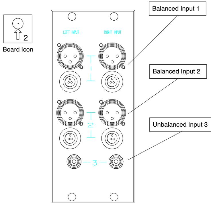
**Figure 6: Spirito Reference Input Card Connectors**
