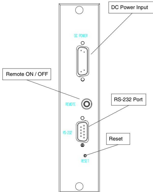
**Figure 5: Spirito Processor Card Connectors**
