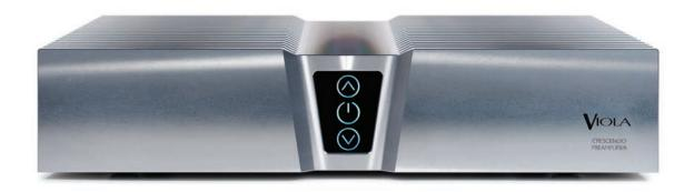
The Viola Crescendo preamplifier is a single chassis stereo preamplifier. The Crescendo chassis is milled from a solid billet of aircraft grade Aluminum. This results in a very rigid chassis with very low resonance. The Crescendo has a prism cut machine finish and a custom Viola anodize finish.
